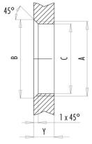
Installation direction: o-ring sits on chamfer.
